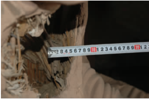
图 2 造像内衬谷杆及织物残留 Fig.2 The remain cornstock and cloth inside
