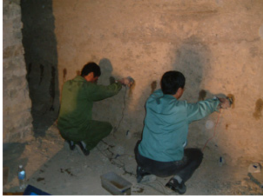
图 6 洞窟内高密度电阻率探测现场 Fig.6 Electrical resistivity measurement in progress
